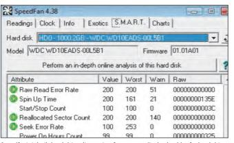
Speedfan's inbuilt hard drive diagnosing feature can display health of a hard drive
